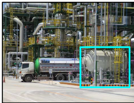
Light Cracker Bottom Drum
